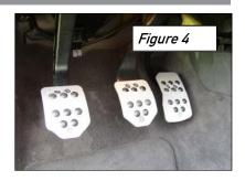
Be sure not to over tighten the bolts for the accelerator, clutch, and footrest covers as the factory pedals and base are plastic.
