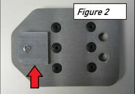
Once you have verified that the pedal covers are where you desire them to be on the pedals, support each pedal from behind and carefully scribe the outline of the bolt hole openings for the covers onto the pedals.
