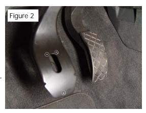
Be sure to place the accelerator cover in a position that allows sufficient space between the brake and accelerator pedals and does not hit the carpet when fully depressed!
