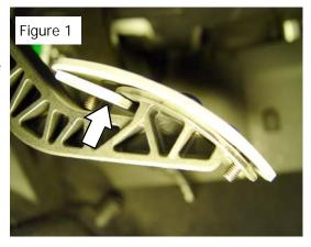
When properly installed, the pedal is sandwiched between the cover and adaptor. Use the enclosed 3/8" Allen head bolts, which thread into the adaptor plate, to temporarily install.
