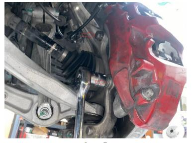
Step 5 Remove the caliper from the rotor and set it aside. Remove the rotor set screw with a T30 torx bit.
