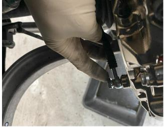
**Step 12** Route the brake line as OE was, making sure the grommets are clipped into their respective retainers.
