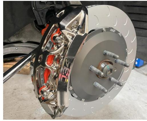
**Step 11** Now that it's sitting on the rotor, align the bracket and wheel knuckle/hub holes. Using the supplied M14 bolts and a 12mm Allen socket, torque to 195Nm.
