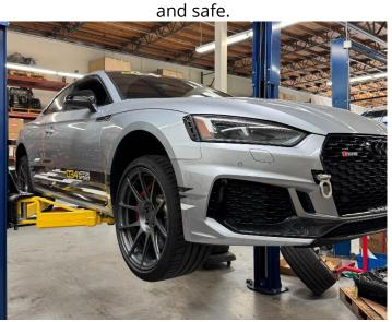
Step 2 Take the wheel off using a 19mm socket on the lug nuts (17mm for OE).
