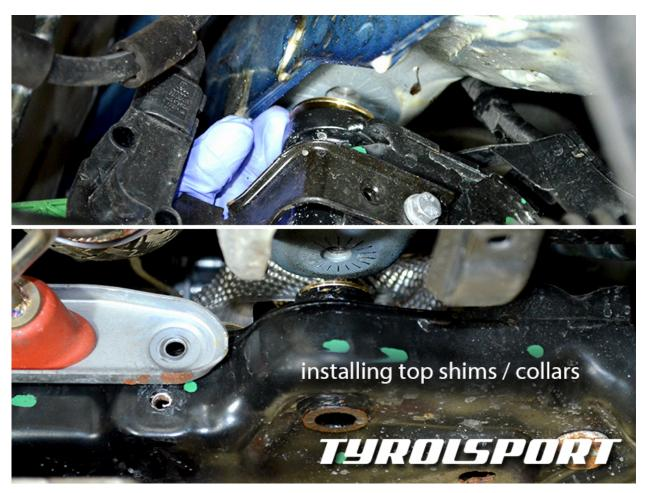
9.) Install the lower collars onto the supplied ARP bolts, using the supplied copper paste on the bolt threads start to thread them in the front position leaving them loose.
