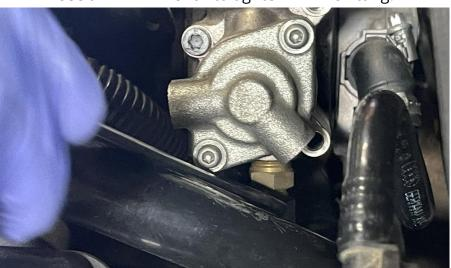
**Step 29**Use a 24mm wrench to install pressure sensor.
