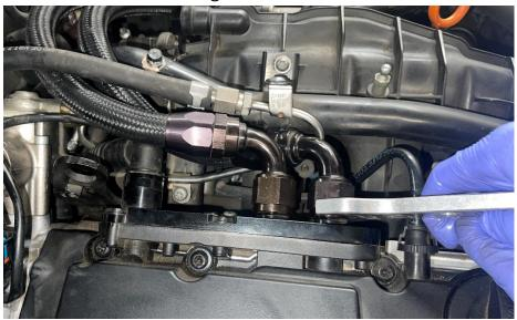
**Step 33**Use a 10mm socket to reinstall bracket.
