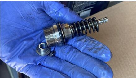
**Step 22** Install the retaining washer on the piston.
