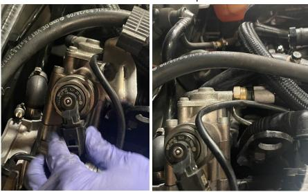
**Step 32**Reinstall/tighten catch can lines.
