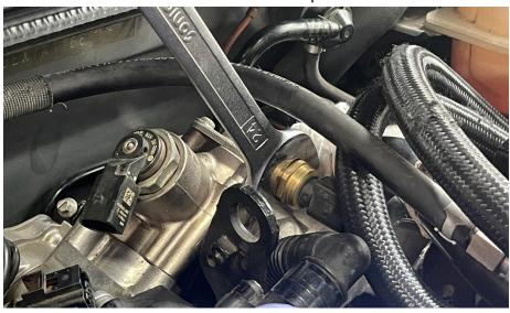
**Step 30**Use a 13mm socket to install bleed screw.
