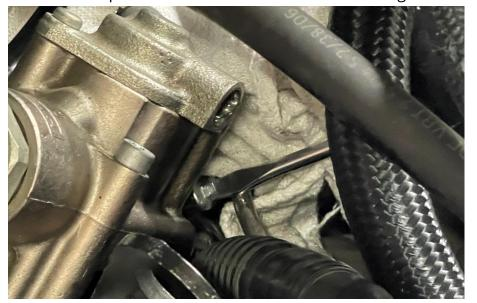
**Step 28**Use a 17mm wrench to tighten HP line fitting.
