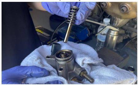
**Step 18**Using an 18mm deep socket, remove the retaining nut.
