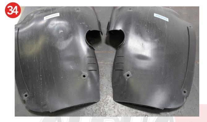
35. Reinstall the wheel well liners and wheels.
