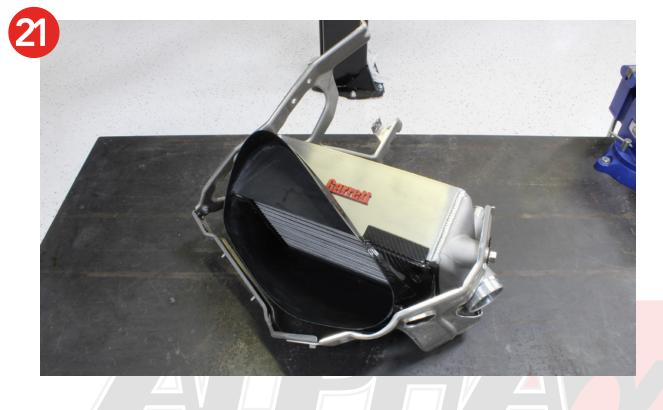
22. Set the upper carbon duct into place on the top of the intercooler. Note the location of the duct where it sit across the weld area. Cut and apply foam stripping to this area.
