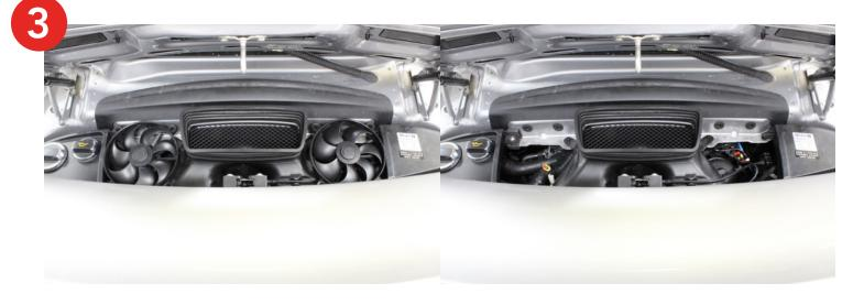
**4.** Remove the corner panels. On the left side corner panel, remove the coolant tank cap. Remove the 10mm bolt from the right corner. Disconnect the hose from the oil fill then slide the panel upwards off its alignment bracket. For the right side corn cover, just carefully pull upwards while wiggling to release the panel pins from the grommets.
