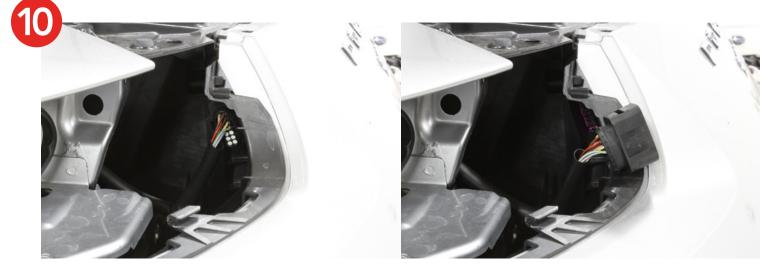
**11.** Disconnect the two connectors located behind the right side taillight. They are contained in a plastic holder.
