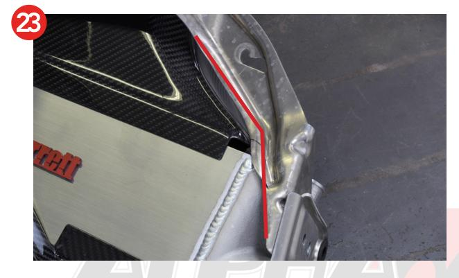
**24.** Before reinstalling the intake duct, you will need to cut off the mounting stud by the top in the picture shown. After trimming, reinstall the intake duct.
