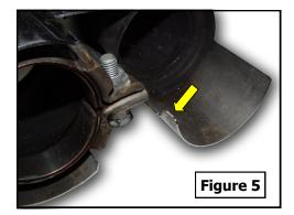
**Please note that the tailpipe sections are side specific.** Decals on the tailpipes indicate their proper locations. Ensure that the tailpipes extend into the tips past the compression rings at the entrance of the tips. If the tailpipes do not extend deep enough into the tips, you will run the risk of the tips falling off during operation.
