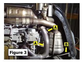
3. Depending on factory build variance, there may be interference between the rear of the AWE Tuning mufflers and a bumper support brace (at arrow B in Figure 3). If there is contact, loosen the brace bolts and rotate the brace until clearance is gained.
