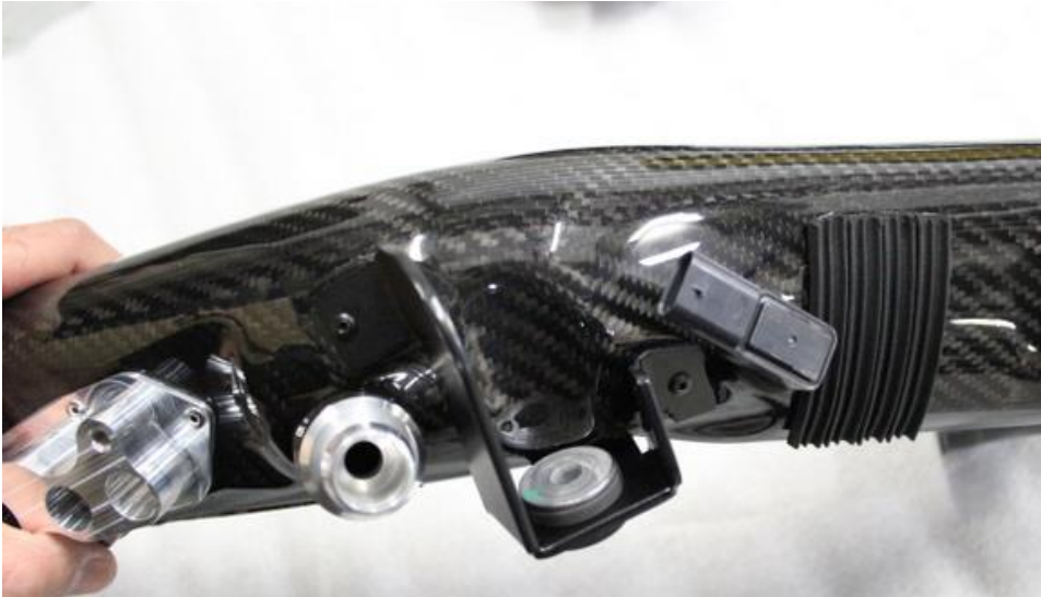
17. Install the MAP sensor and angle it as shown. Also install the rubber mount with the metal insert into the bracket.
