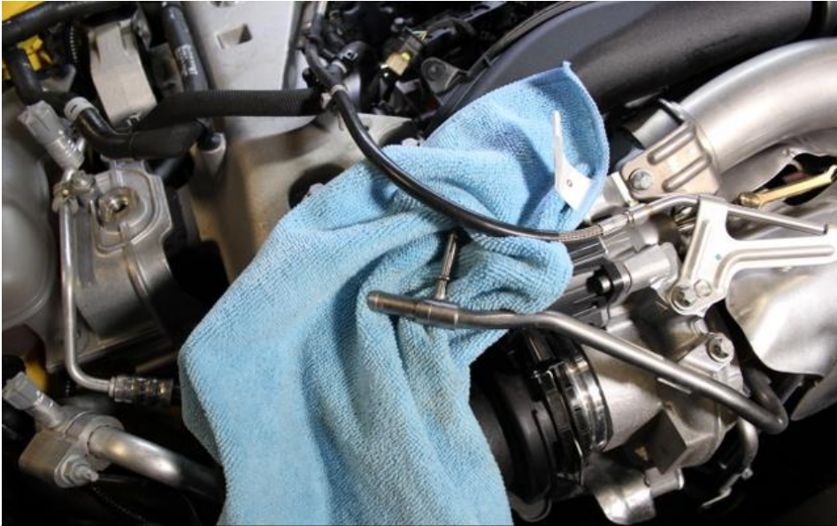
13. Put a cloth underneath the exposed metal coolant pipes to protect the tube.
