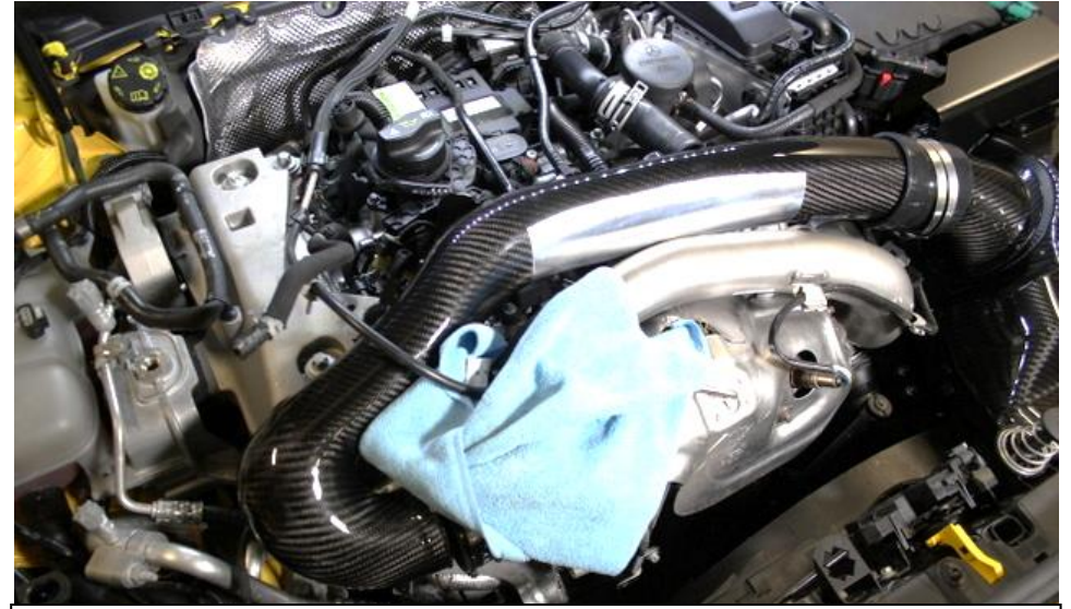
22. Carefully slide the tube into position – make sure the cloth is still covering the exposed metal coolant tubes.
