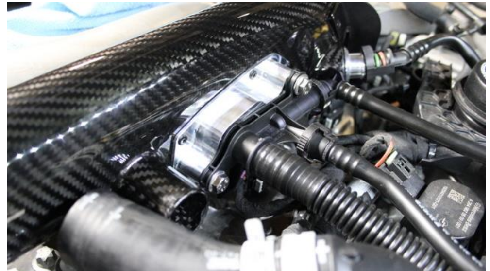
26. Push the breather block into the machined block and secure with the supplied M6 bolts.
