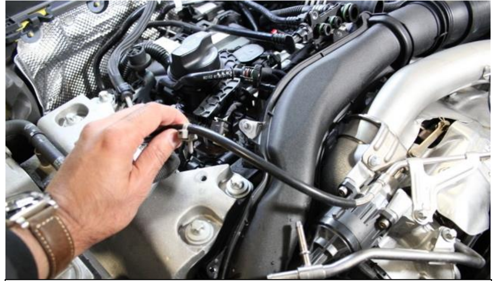
10. Pull this cable clip out for more space to remove the tube.
