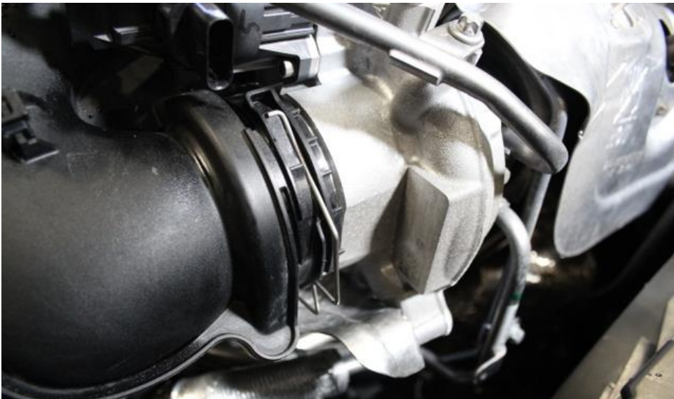
11. Pull the wire clip out which secures the tube to the turbo.
