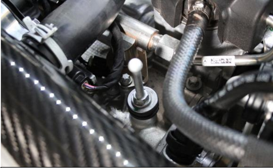
29. Install the remaining original bolt on top of the rubber mount as shown.
