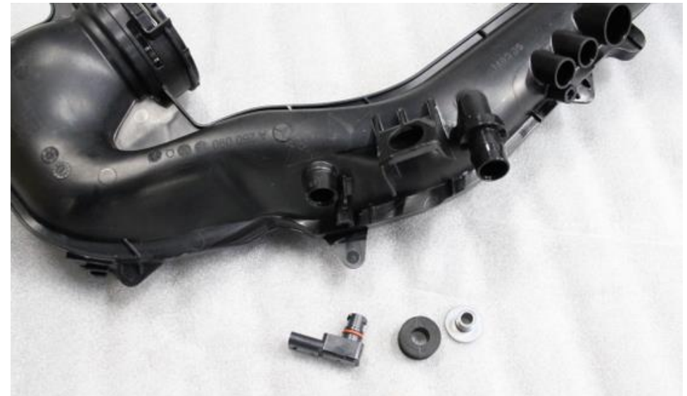
16. Remove the MAP sensor by rotating it 90 degrees and pulling out. Also remove one of the rubber mounting grommets.
