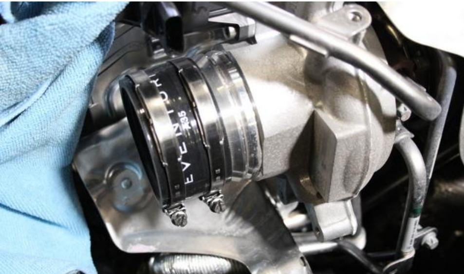
19. Push the silicon onto the turbo – notice the position of the clamps. If you have an A250 please use the supplied reducer which has A250 marked on it.
