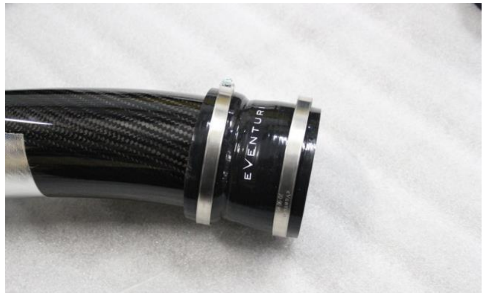
20. Insert the larger silicon hose onto the airbox side of the tube as shown.
