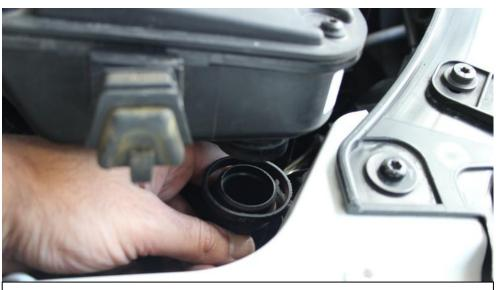
10. Disconnect breather tube from the airbox by pinching in two side of the flange around the tube to release the clips. The airbox can now be pulled upwards and removed from the engine bay.
