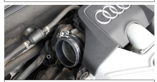
12. Push the smaller silicon coupler over the throttle body. Ensure it is fully on and uniform all the way around. Use 2 x 70-90mm hose clamps as shown and secure the hose clamp around the throttle body.
