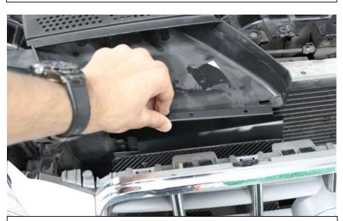
31. Place the scoop assembly into position so that the 3 slots on the metal scoop extension sit over the stock duct edge.
