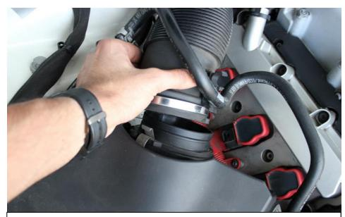
9. Remove the inlet tube from the airbox side too and completely remove from the engine bay.
