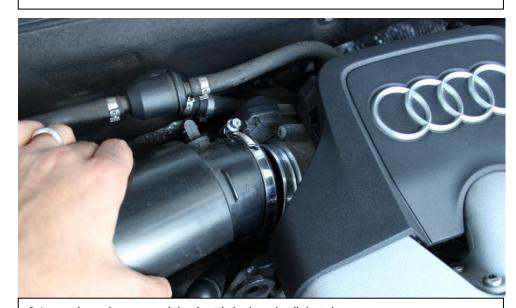
8. Loosen hose clamp around the throttle body and pull the tube away.
