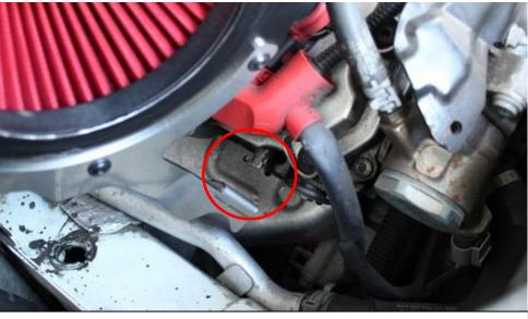
18. The flange on the bracket needs to line up with the mounting point where the earth cable was attached.
