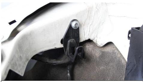
11. Remove this bracket which held an airbox mount. Retain the screw for use later on.
