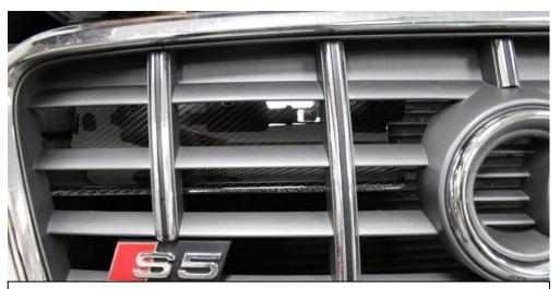
36. Position the scoop so it sits against the grill – avoiding any obstructions. Once in position, mark and drill 3 holes in the stock duct through the 3 holes on the scoop using a 5mm drill bit. Do not secure the scoop to the duct yet.
