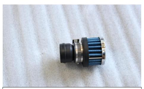
51. Push the breather adapter into the small filter and secure the clamp.
