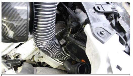
44. Feed the flexible tube underneath the headlamp - see next step.
