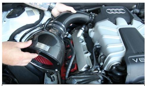
17. Push the intake tube into the silicon hose at the throttle body. Do not secure fully yet – tube should still be able to rotate freely.
