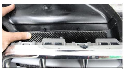
35. Place the carbon scoop by itself onto the duct as shown.
