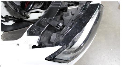
42. Now carefully move the headlight out by a couple of inches. Just enough to allow the flexible duct to be positioned.
