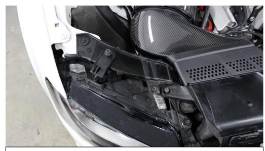
50. Now carefully push the headlight back into position and secure the 3 previously removed screws.
