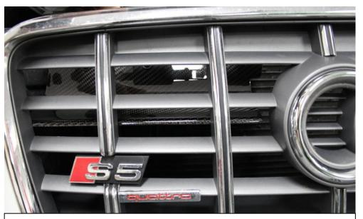
32. Position the scoop so it sits against the grill – avoiding any obstructions. Once in position, mark and drill 3 holes in the stock duct as shown in next step.
