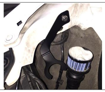
52. Push the breather assembly onto the secondary air pump tube – it will click into place. Also secure the breather filter bracket to the chassis using the previously removed screw in step 11.
