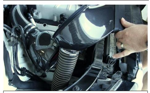
43. Take the duct assembly and lower the flexible tube behind the headlight.
