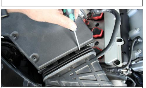
3. Using a screwdriver – carefully release the rubber duct from the airbox by pushing down the tabs.
