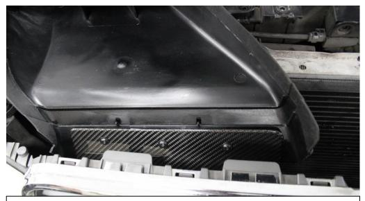
48. For the pre-face lift version, lower the scoop into place and secure with 3 black screws and lock nuts.
