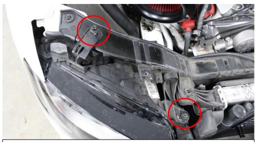
40. The flexible tube will sit underneath the headlamp – for ease of installation, we will move the headlamp forward. Remove the 3 screws holding it in place. 2 Shown here.
