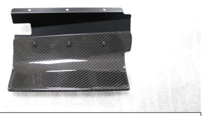
30. Assemble the scoop to the metal scoop extension plate using 3 black M5 screws and lock nuts
