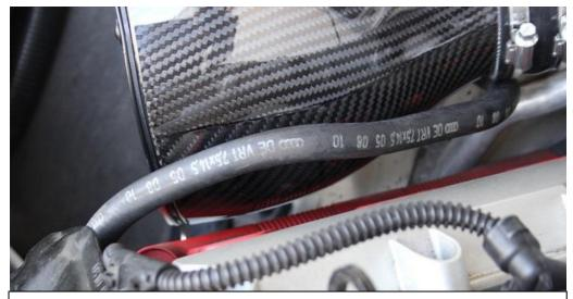
25. Looking at the housing from the side – there should be a small gap between the housing and the engine. Adjust the position of the housing and secure the M6 bolt on the bracket.
