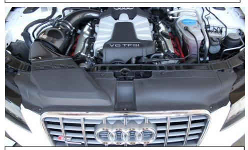
$55. \ In stall \ the \ slam \ panel \ cover \ and \ secure \ with \ the \ screws/plugs \ previously \ removed.$
