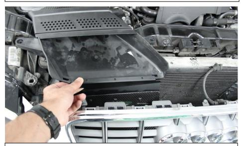
47. Now position the scoop assembly over the holes previously drilled and secure with 3 black screws and lock nuts. Photo shows facelift version.
