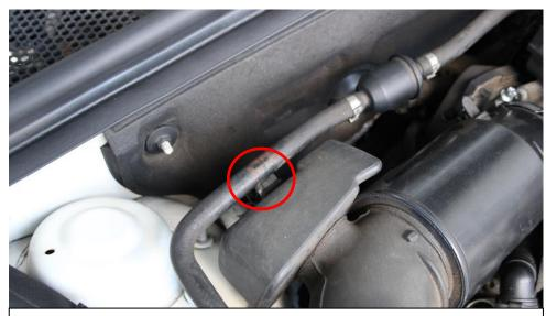
6. Remove the hose at the rear from the silencer box on the tube.
