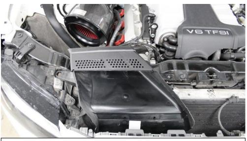
34. For pre-face lift S5's: Place the stock duct in place and secure with the 2 screws previously removed.
