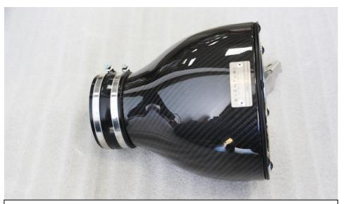
13. Push the larger silicon hose onto the filter housing. Use 2 x 80-100mm hose clamps as shown and secure the hose clamp around the filter housing. Leave the other loose.
