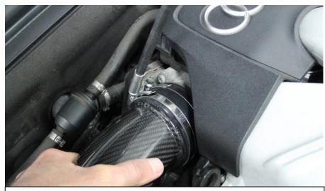
26. Now push the tube into the silicon so that the carbon flange meets the silicon uniformly and tighten the remaining hose clamp – don't over tighten.
