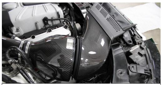
46. Keep pushing the flexible tube down until you can line up the carbon duct with the carbon housing. The metal cowl at the mouth of the filter should go inside the carbon duct. Be careful not to pull the rubber edging on the duct out of position. If this does happen – pull the duct back out and re-align the rubber edging.
