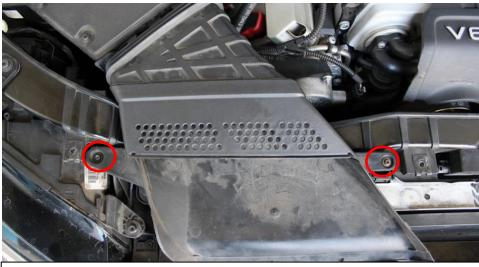
2. Remove the 2 screws holding the intake duct in place.
