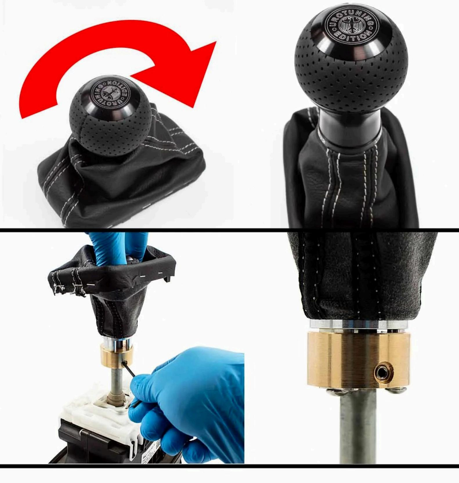
5. Pull the shift knob with trigger mechanism up to its highest point and secure the bolts evenly.
