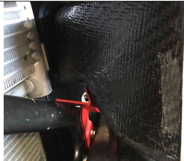
38. Now secure the bracket to the brace by using the supplied M6x20 bolt and lock nut (see step 24). Bracket shown in red for illustration. Push the grill back into the bumper.
