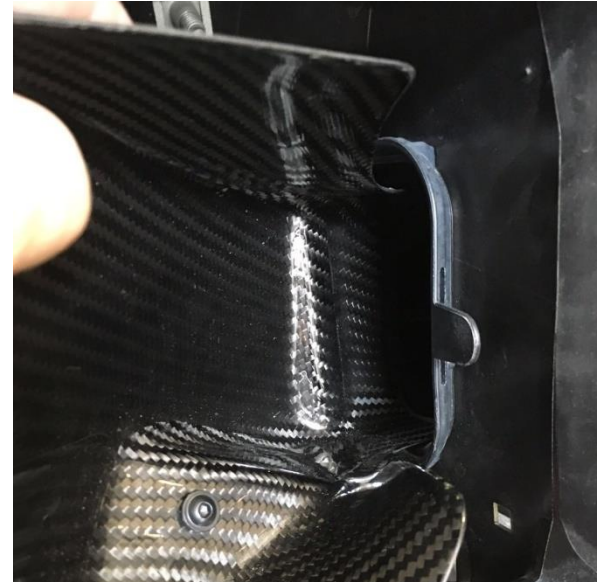
36. Push the scoop down so that it locates inside the stock duct as shown. Your scoop installation is now complete. Push the grill back into the bumper.
