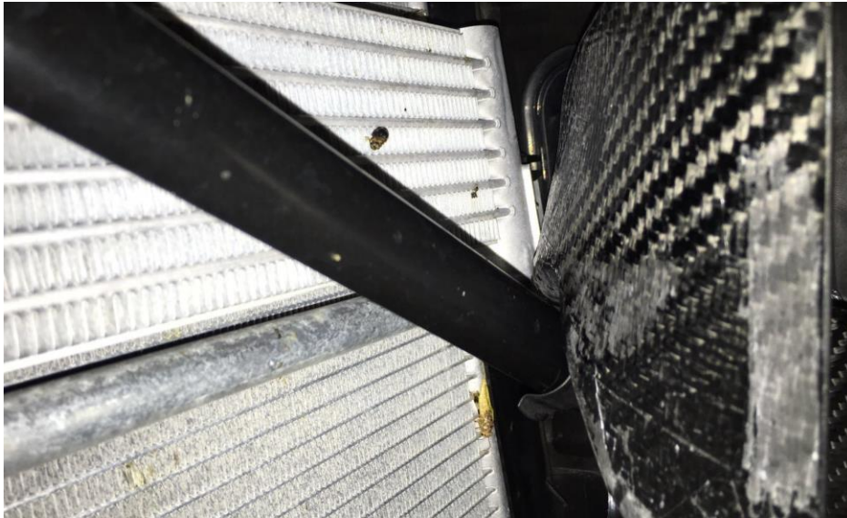
35. For the M235i and M135i, push the clip on the back of the scoop onto the metal brace bar behind the grill.
