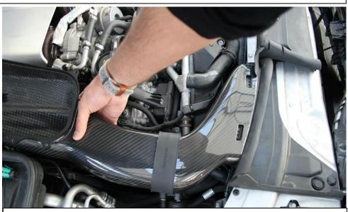
4. Install the airbox base by pushing the duct into position and then rotating it down to push the rear mount into place.
