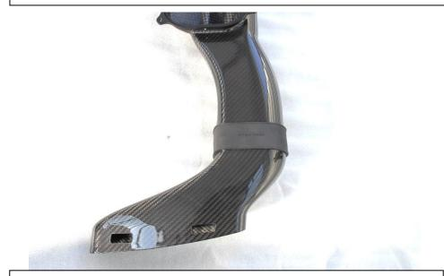
3. Push the corresponding carbon duct into the EPDM coupler.
