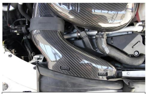
5. Adjust the duct position if required by pulling it towards the slam panel. The duct should sit as far forward as possible.
