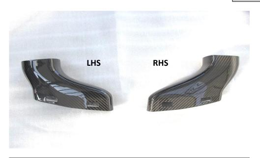
1. Identify the LHS and RHS Carbon Ducts as shown. The 2 rectangular holes should be facing upwards.
