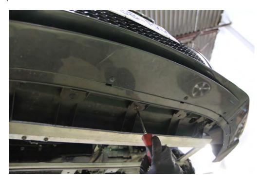
**Step 3**: Remove the 5x T25 Torx, 1x T30 Torx and 1x 10mm nut holding the inner fender lining to the car. Repeat for the passenger side of car.
