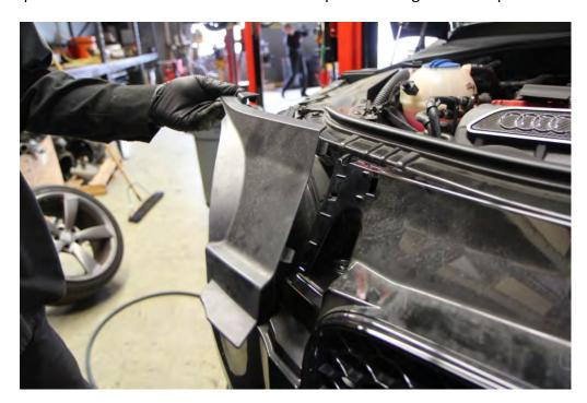
**Step 7**: Remove the 4x T30 Torx screws attaching the top of the bumper to the rad support.
