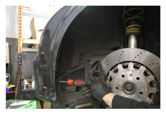
**Step 4**: Pull back the upper fender liner and remove the 2x 10mm nuts holding the bumper to the rad support. Repeat for the other side of car.
