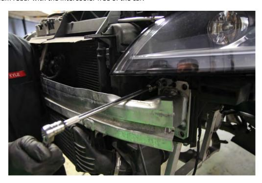
**Step 17**: Remove the 1x T30 Torx screw holding the horn bracket to the rad support. Remove both horns off the factory mount and attach to the supplied CTS bracket using the factory nuts. Reattach the CTS bracket to the car using the T30 Torx screw.
