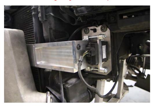
**Step 21**: With the silicone clamps tightened, proceed to tighten the 4x 6mm bolts holding the intercooler mounting tabs to the rebar. Tighten the 8x 10mm triple square bolts. Attach the temp sensor bracket to the billet rebar using the 6x16mm button head screw and push the sensor into place.
