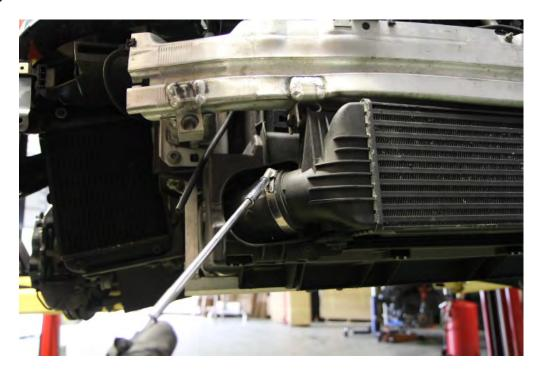
**Step 16**: Remove the 8x 10mm triple square bolts holding the rebar to the frame. Pull the aluminum rebar with the intercooler free of the car.
