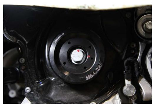
**Step 7**: Utilize your counter holder tool and long handle breaker bar with the 24mm socket to torque the bolt a ¼ turn further. With your two marks aligned, the pulley is installed.
