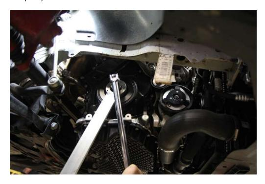
**Step 6**: Install the new lightened pulley taking care to **align the spines** on the back of the pulley in the correct position. This is critical. Install the supplied **new** OEM bolt. Utilizing your torque wrench with the counter holder tool, torque the bolt to **110 ft/lbs**. Use a marker to make a 12 o'clock mark on the bolt and a 3 o'clock mark on the pulley.
