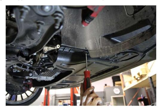
**Step 2**: Remove the passenger side wheel then remove the 6x T25 torx screws holding the passenger side lower inner fender liner to the car. Pull the liner free of vehicle.
