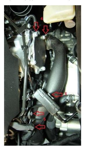
Step 7: Remove the rubber turbo outlet pipe coupler. Move the outlet pipe out of the way (having a friend help is good).
