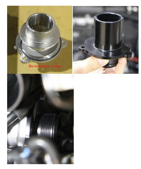
Step 10: Reinstall factory coupler, align the coupler as shown and tighten clamps. Reinstall turbo outlet pipe, DSG breather (if equipped) and air intake.
