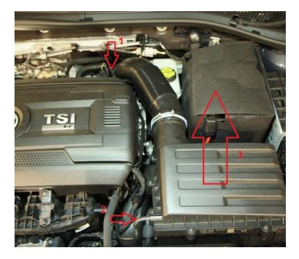
Step 4: Remove two 7mm clamps on the turbo outlet.
