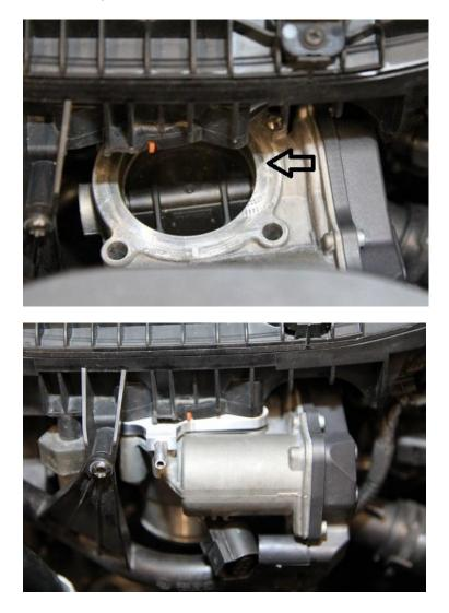
7. From bottom of car, reinstall and tighten 4x T30 torx screws. Torque screws to 7 Nm (5.2 ft/lbs).
