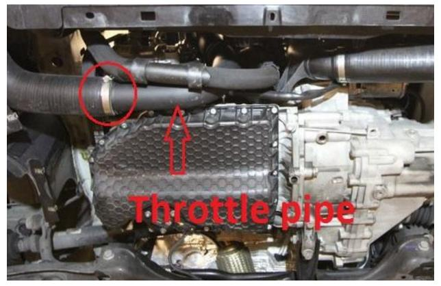
4. From bottom of car remove 4x T30 bolts holding throttle body to intake manifold. Long extension helps (approx 24" worked for us). Do not remove throttle body completely off the vehicle. Make sure the factory orange o-ring remains installed in the intake manifold.
