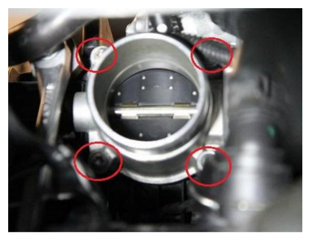
5. On the intake manifold, trim off the locating tab to allow for boost tap clearance. This is easily done with a sharp knife or a hacksaw blade.
