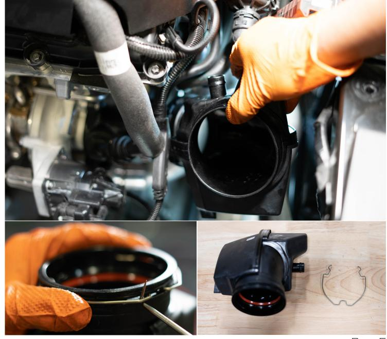
HIGH-FLOW TURBO INLET PIPE FOR 858C
