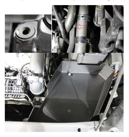
Step 5: Attach the silicon coupler to the turbo inlet, install grommet into the bracket on the intake tube and install tube. Secure hose clamps and push the grommet onto factory mounting stud. Connect valve cover breather to intake tube using supplied silicon hose.
