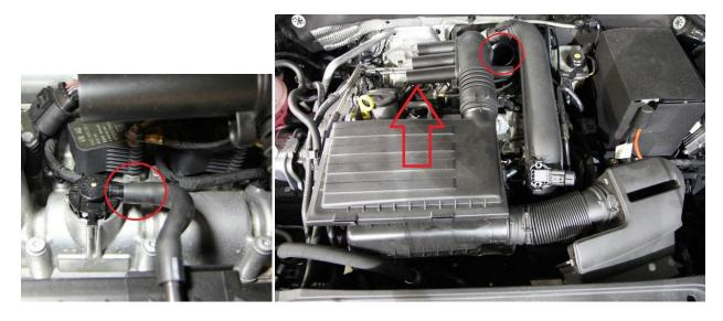
Step 4: Assemble 6 small bolts (philips+7mm socket) into the heatshield, attach the rubber strip to the front of the heatshield. Relocate the smaller coolant hose next to the main hose as shown in photo. Secure heatshield in place with M6 flanged bolt (10mm socket).
