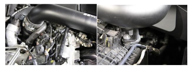
Step 6: Install air filter and ensure that intake tube does not hit the heatshied. Readjust if necessary. You are done!
