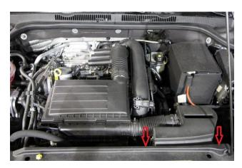
Step 2: Remove the clamp holding the intake to the turbo inlet.
