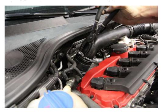
**Step 8:** Pull the entire airbox assembly out of the engine bay.
