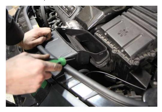
**Step 3:** Pull upwards on the engine cover to remove.
