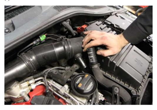
**Step 5:** Use your 5mm socket allen to undo the lower right side mounting bolt.
