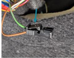
Once the terminals slide all the way in, squeeze the connector hinge in (shown in the right picture above in the open position). This hinge will only close if the terminals are all the way in.
