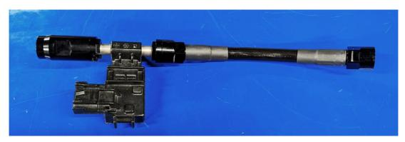
C. Now, slide the hose end of the assembly onto the chassis fitting first. Then slide the adapter fitting onto the HPFP hardline by slightly bending the hose. Do not force any of these connections on. They will slide freely onto the car's barbs.
