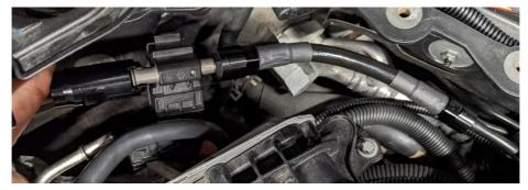
D. Once the assembly has been slipped onto each of the car's barbs, simply thread the blue nuts onto each fitting and tighten them down with a 19mm wrench
