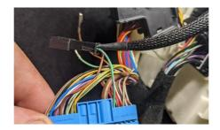
21. You will now have two loose wires on the car's harness (previously removed from the blue connector). Slide these terminals into the small black Dorch supplied connector. Slide the terminals in with their locking tabs facing up towards the hinge on the connector (left picture below). The connector is marked for position 1 and 2.
