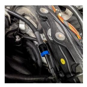
3. Pull the other end of the hose up on top of the intake manifold (pictured) to attach both hoses to the ethanol sensor. For the sensor fittings, you will need to slide the nut on the sensor first (via the nut's slot) and then push the hose onto the sensor. Take note of the orientation of the sensor:
