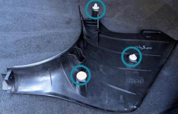
14. Next remove the module cover. There is one T20 Torx, followed by two clips. The clips only have latches on the outer tangs. Push in each outer tang with a screwdriver and pull out to remove the cover:
