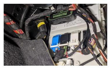
At this point, the installation is complete. Zip-tie any excess sensor harness length up and out of the way neatly. You now have a fully reversible plug and play ECA that communicates directly with the DME. The parts can all be reinstalled in reverse order and the battery can be reconnected. Once everything is buttoned up, you will need to make sure you are running the appropriate software via MHD, BM3, or Ecutek.
