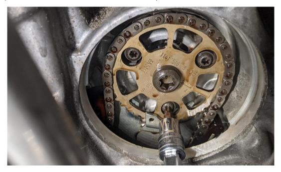
16. Now using a flat head screwdriver, very carefully depress the timing chain tensioner (pictured on the left below). Hold the screwdriver in place and then slide the timing gear off the tip of the Vacuum pump shaft. Once the gear is off the shaft, release the screwdriver and allow the gear to rest as pictured (right):
