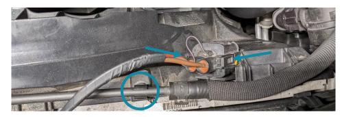
6. Remove the T25 fastener from the upper corner of the fan assembly and release the second clip for the coolant line:
