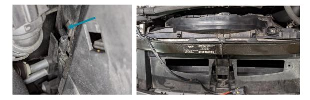
Be sure to lift up slowly with electrical harness and coolant line moved out of the way. Watch for any snags on any other hoses on the lower sections of the fan as it lifts out.
