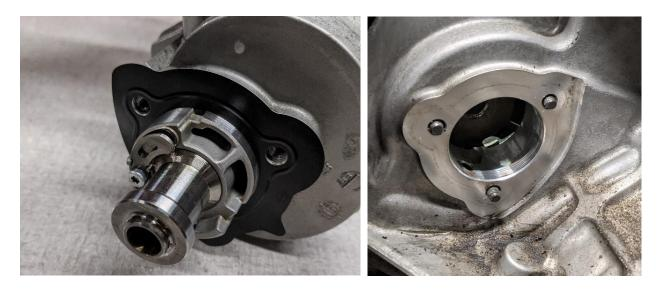
21. The Dorch Engineering vacuum pump assembly can now be installed in the block. Once it is seated in place, the timing gear needs to be placed back on the front of the shaft (reverse process of Step 16). This will require carefully using a screwdriver (again) to hold back the timing chain tensioner while the lining up the gear onto the front of the shaft.
