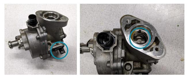
19. Now transfer the cam follower and cam sensor (with O-ring seal) on to the Dorch Engineering supplied vacuum pump assembly. Make sure the follower is oiled when it is dropped into the new assembly.
