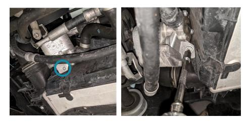
3. Next remove the front half of the fresh air inlet via 2x push pin clips and 2x T25 fasterners:
