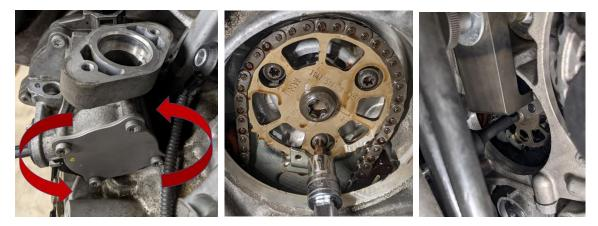
23. Now, reinstall the timing gear lock tool and tighten the center T55 bolt to the final torque.
