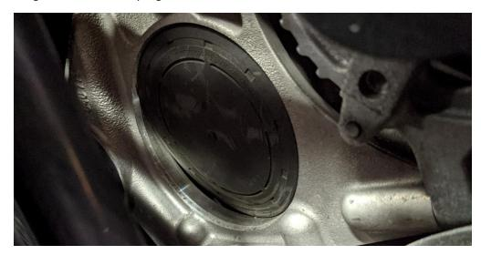
The goal is to push the bottom of the seal in far enough so that the top edge pops out. This sometimes doesn't pop out easily and may require careful usage of hand tools such as hooks and SMALL rounded pry bars. Be extremely careful not to gouge the sealing surface or to push any tools too far into the timing assembly.
