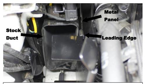
15. Look into the cavity towards the front of the car and you will see the stock duct opening. The leading edge of the new shield must go between this duct and the metal panel next to it as shown. Once positioned, push the shield in-between this gap.
