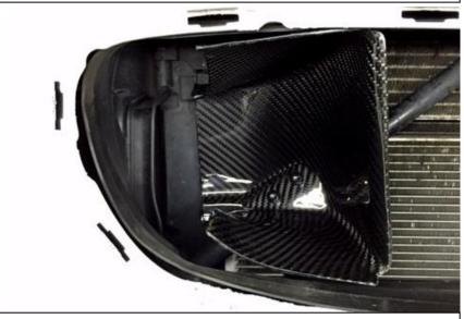
38. Now slide the scoop downwards so the lower carbon flap meets the rubber trim as shown in the next photo.
