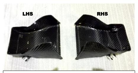
34. Identify the LHS and RHS scoops as shown. The clips should be at the bottom.
