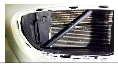
35. Starting with the LHS Scoop – look into the left side of the bumper. The clips on the back of the scoop will secure onto this strut brace.
