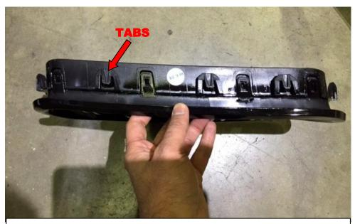
33. Pull the bumper cover out to gain access to the top of the grills. You will see tabs which need to be pushed in using a screwdriver. Pull the grills out while pushing these tabs in. You can pull the bottom tabs up with your fingers.
