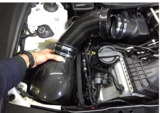
26. Now turn the Carbon tube downwards and into the silicon coupler as shown. Loosen the hose clamp around the silicon if required.
