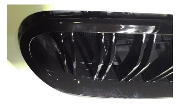
39. Carefully push the grill back into place. The lower flap of the scoop should go underneath the grill. Use your fingers to ensure it does as you push the grill in. At the same time, the upper flap of the scoop should go above the grill as can be seen in the next photo.
