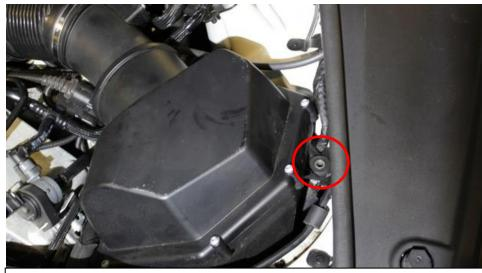
2. Starting from the right hand side remove the Torx screw securing the airbox in place as shown.
