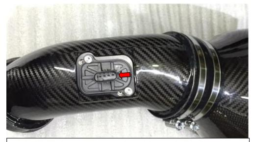
24. Remove the MAF sensors from the stock airboxes and install them onto the new tubes. **Make** sure they are oriented correctly – there is an arrow on them to show airflow direction as highlighted here in red. Secure them with the provided new M4 Torx screws.
