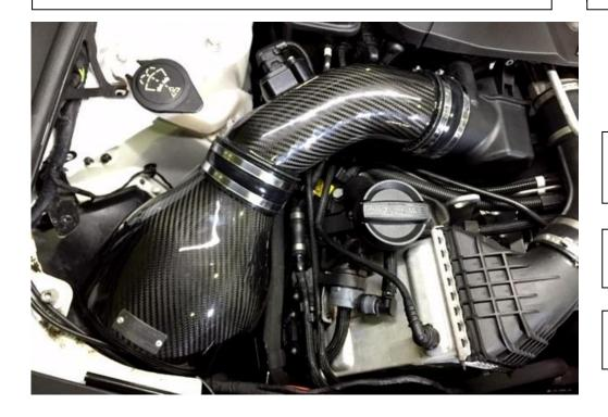
29. The MAF sensor mount should be at the back of the tube as shown – insert the MAF plug back into the sensor. Push it in fully. Now tighten all the hose clamps. Ensure the housing is pushed up into the tube fully and the tube is pushed into the turbo inlet fully.
