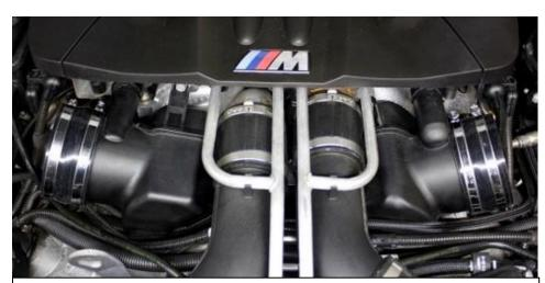
20. Push the 83mm silicon couplers over the turbo inlets as shown. Push them on fully and tighten the first hose clamps on both sides to secure to the inlets. Ensure the clamps are straight. Leave the outer clamps loose.
