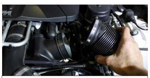
8. Now loosen the other hose clamp on the inlet tube and remove tube completely. Repeat this process for the Left Hand Side to remove the airbox and inlet tube.
