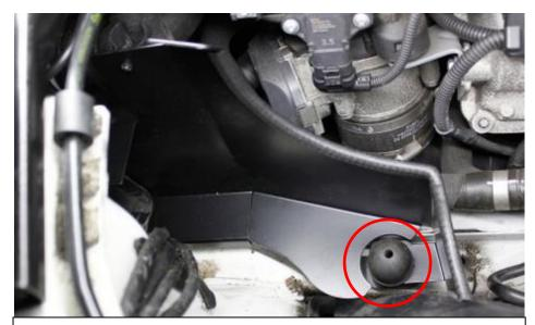
17. Now secure the shield with the rubber grommet previously removed. The shield will still have some movement – this is required.
