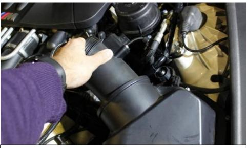
6. Pull the airbox upwards from the tube to release it from the push fit mounting points. Be careful to move any pipes out of the way. The airbox can be completely removed from the engine bay.
