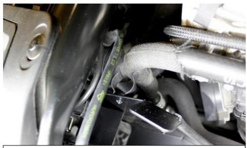
18. Finally secure the stock rubber hose into the clip on the side of the shield. Repeat this process from step 14 for the other side.
