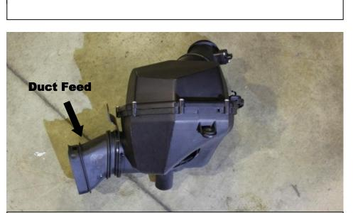
7. The complete airbox should look like this – complete with the duct feed.
