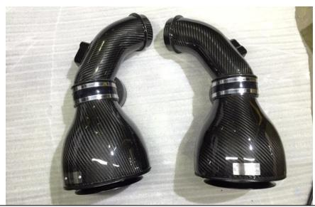
23. Now take the Carbon filter housings and push them into the silicon couplers. Do not tighten the clamps yet.
