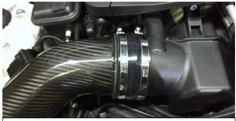
27. Ensure the tube is fully inserted into the silicon coupler. The carbon flange should be up against the silicon all the way around.
