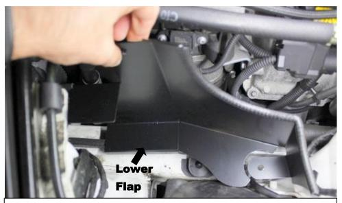
14. Starting with the RHS shield, place it in the right hand cavity, position the lower flap over the rubber edging previously inserted.
