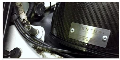
28. There should be adequate clearance between the housing and the front panel. Since the clamps are still loose – you can rotate the tube and the housing until you have good clearance.
