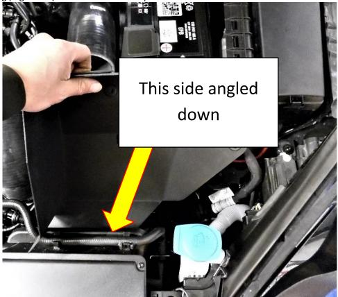
6. If you have a non-OEM inlet hose installed, loosely attach the hose clamps to the end of the silicone intake hose. If you are using the OEM inlet hose loosen the clamp with long nose pliers or a hose clamp removal tool. Take the alloy intake pipe and insert the longer end into the silicone intake hose through the rubber O-
