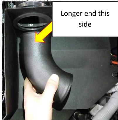
7. Fit the Forge filter onto the end of the alloy pipe and secure it into place with the remaining 70-90mm hose clamp. Angle the filter so that it has between 10mm-15Mmm clearance from the bottom the filter tray and pay attention to the radiator hose so that nothing is fouling the filter. Use a 7mm socket and suitable drive, long nose pliers or a hose clamp removal tool to tighten the clamp depending on what inlet hose you have installed.
