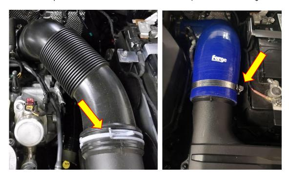
2. Pull with a sharp motion to remove the Vac line from the front right side of the engine, the other end will connect to the airbox which you can leave attached.
