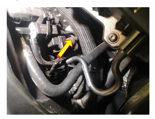
3. The airbox is located by rubber grommets on three pins. Rock the airbox left to right while pulling in an upwards motion to remove it.
