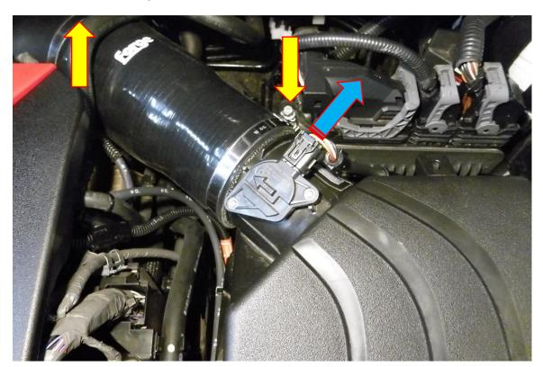
3. Disconnect the vacuum hose from the airbox, and from the airbox pump.
