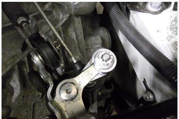
10. To lock the nut into position, use the supplied split pin. Make sure the split pin passes through two of the groves in the FMSS5 nut and through the hole of the gearbox linkage pin. You may have to adjust the nut, so it lines up.
