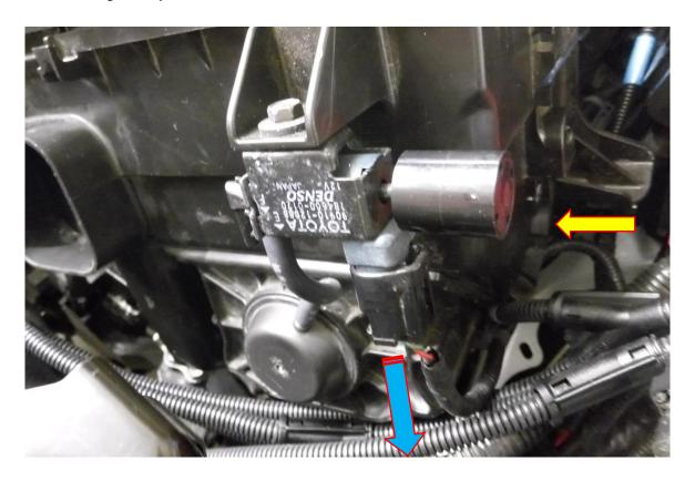
5. Locate the gearbox linkage and remove the retaining pin. Pull the gear shift rod from the linkage.
