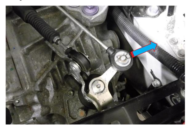
6. Insert the shifter pin and M8 nut into the FMSS5 body as shown in the picture below, adjust the shift pin back and forth until the desired position is found. Use a 16mm spanner to secure it place.
