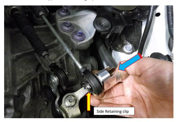
8. Mount the FMSS5 and gear shifter rod in situ onto the gearbox linkage. Place it underneath and push it upwards as far as possible.
