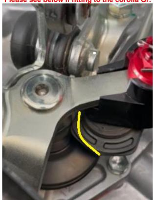
Using a Dremel or suitable tool remove the corner of the shifter cable plastic mount to the yellow line as pictured above this will enable you to have full adjustment of the Forge Motorsport FMSS5.
