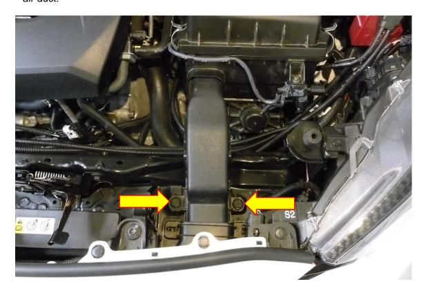
2. Using a 7mm or 10 mm socket and ratchet loosen both hose clamps of the inlet hose which will allow you to remove the hose from the airbox. Press in the retaining tab on the MAF loom and unplug it from the MAF.
