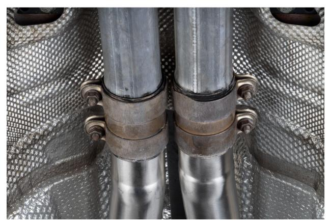
Ensure the Mid Pipes are situated properly, then tighten exhaust clamps, and downpipe nuts.
