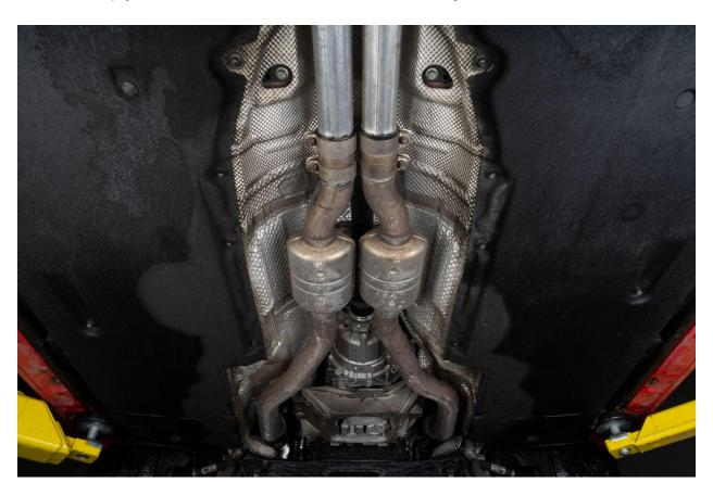
Remove six 12mm nuts from the Downpipe side of Mid Pipes. Accessing top bolt requires extension and swivel socket.
