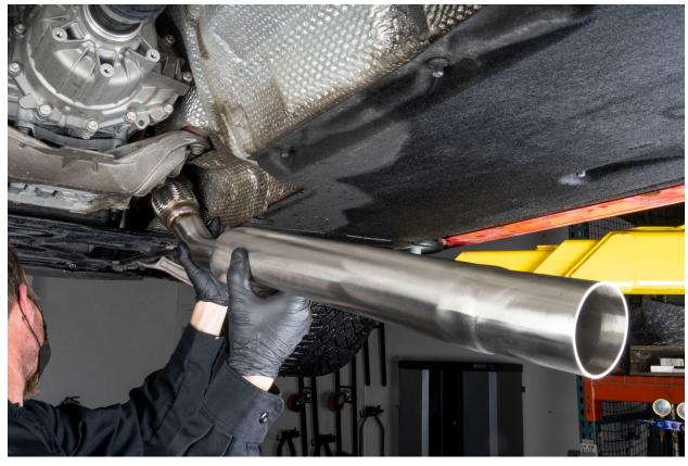
Position Mid Pipes into the rear exhaust clamps.
