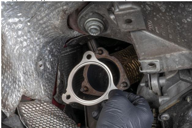
Position IE midpipes onto the OEM downpipe studs then finger thread nuts to the downpipe bolts.
