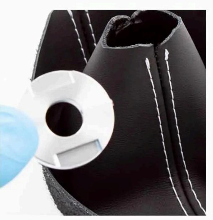
All BMW/MINI models and models and models shift boots with 3 or more seams: use the flat side of the adjustmentring facing upwards.
