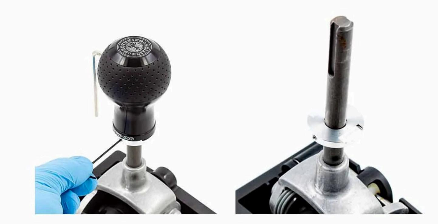
3. Place the shift boot over the rod on top of the adjustmentring. Shift boots with 1 or 2 seams; make sure the seams are centered in the slots of the adjustment ring.
