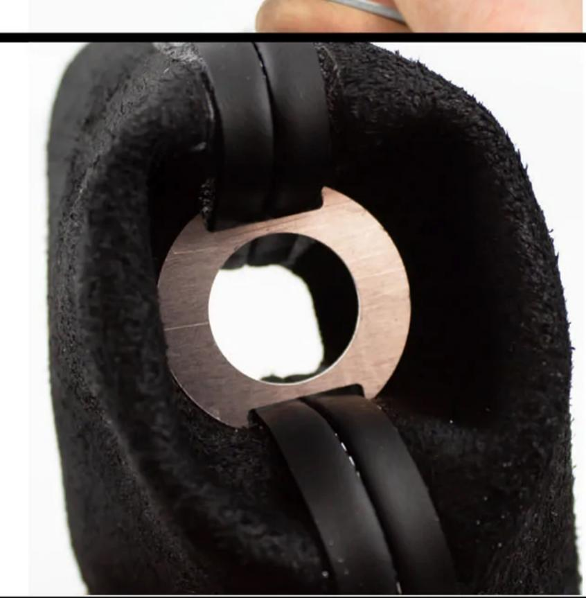
5. Mount the shift boot back in place. Make sure the boot sits free from the threading of the adapter before screwing the shift knob on. If the shift knob does not end up aligned in step 6, it is likely the boot is somewhere in between.
