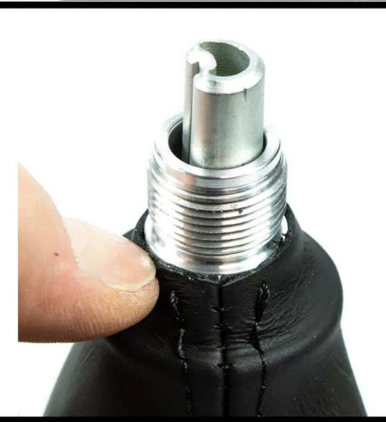
6. Finally, screw the shift knob on.
