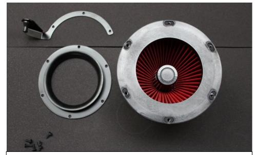
2. Remove all screws and remove the bracket and curved cowl.
