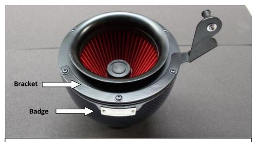
1. First we need to swap the curved cowl with the supplied flat cowl. make note of the position of this bracket with respect to the Eventuri Badge. Take a photo for easy reference. You will need to reinstall the bracket in the same position.
