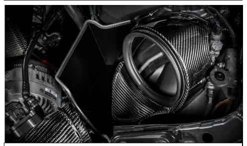
4. Install the new sealed duct in the same way as the original metal duct and secure with the 2 push rivets. Once secured – re-install the tube and filter housing assembly. You can follow the same guide as the original N55 installation guide found on our website in "downloads".
