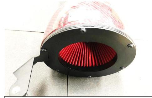
3. Now use the new flat cowl and re-install with the bracket. Make sure the bracket is in the same position with respect to the Eventuri badge.
