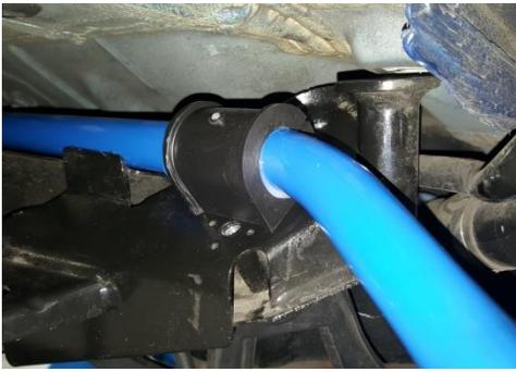
15. Apply supplied grease to inside of supplied urethane bushings and install on NM anti-roll bar.
