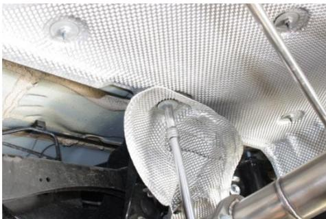
8. Unbolt [1] 10mm hex nut from exhaust heat shield that connects from sub-frame to uni-body.
