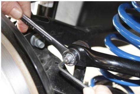
4. Remove upper end-link nut from anti-roll bar by securing stud with T30 Torx or 4mm hex key wrench and loosening nut with 16mm wrench. Repeat for other side.
