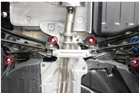
9. Remove the (4) sub-frame mounting bolts using E14 Torx or 7/16" socket. Supporting sub-frame not required.
