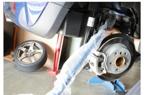
14. Install NM anti-roll bar in reverse of removal of original bar being careful getting around brake lines. **HINT:** Leave plastic wrap on bar to protect finish of bar during installation through sub-frame then remove.
