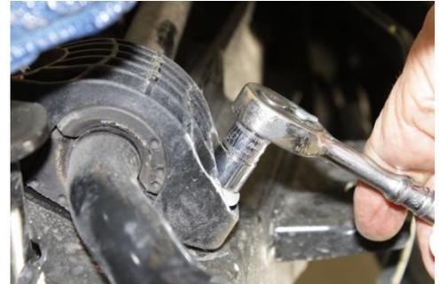
11. Remove the [2] bushing clamp mounting bolts using an E12 Torx or 3/8" socket. Remove clamp. Repeat for other side.
