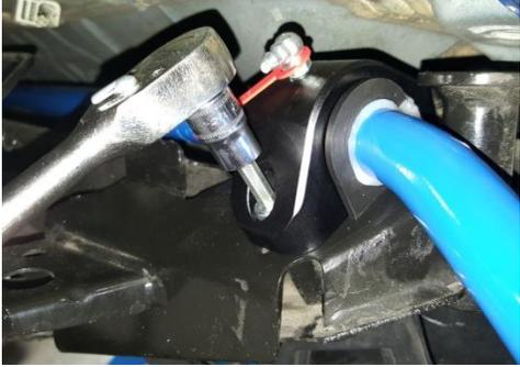
16. Install NM Billet Bushing Clamps (grease fitting facing rearward) and supplied bolts. Torque to 34 Nm (25 ft-lbs).
