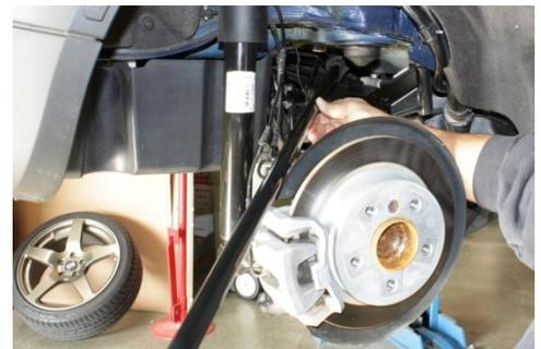
13. Now from right side of vehicle completely remove original bar.
