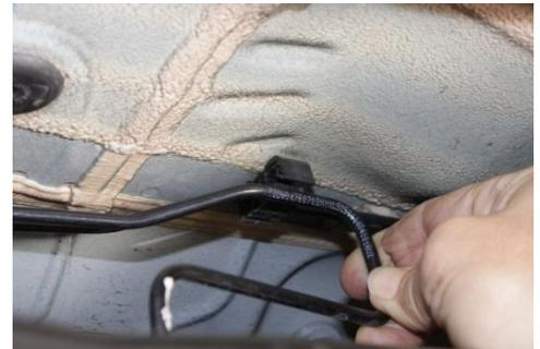
10. **NOTE:** Brake lines will unclip from their support mounts on the uni-body.
