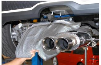
Lower and support exhaust system just enough to unbolt and remove rear muffler heat shield from vehicle, (3)10mm hex nuts and (2)10mm hex bolts.
