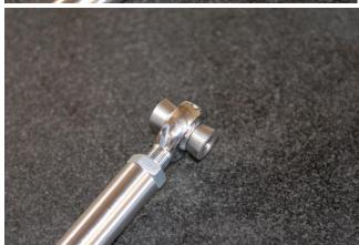
Install supplied stainless steel spacers into ball joints. **NOTE:** The NM Control Arms have been pre-set to the factory length of 20 15/16".
