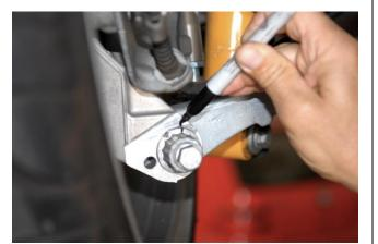
4. Mark existing location of factory adjusting plate to trailing arm on outer control arm bolt with marking pen.
