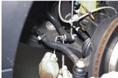
Unbolt nut from anti-sway bar to end link using a 16mm wrench and 5mm hex key wrench. Repeat for other side. NOTE: To ease removal spray threads with WD-40 and then break nuts loose first using a 16mm socket.
