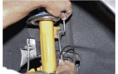
5. Unbolt end link from strut mount using a 16mm wrench and a 5mm hex key wrench, then remove end link. Repeat for other side.
