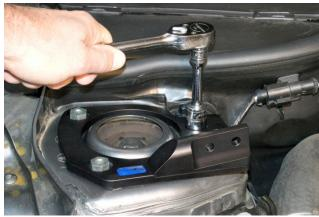
Mount and evenly tighten the NM base plate to strut towers using special long-reach nuts – torque to 34 Nm (25 ft-lbs.).
