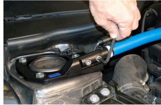
Install and tighten all [4] M8 x 20mm hex socket bolts using a 6mm hex key wrench.
