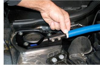
Now hand tighten locking collar on each side of tie-bar. Installation is complete.
