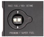
14. NM Power Module has (2) position power switches accessible from the back side. Remove plastic cap to access. DOWN position for Premium fuel 91+ octane (3PSI increase) and UP position for 100+ Race fuel (5PSI increase). NOTE: BOTH SWITCHES MUST BE IN THE SAME DOWN OR UP POSITION.
