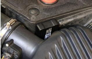
NM Power Module can be mounted in a couple of desired places. With supplied Velcro; either stick right on top of battery cover or on front of battery box.
