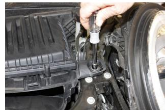
Remove the 10mm hex bolt located on driver side of air filter box.
