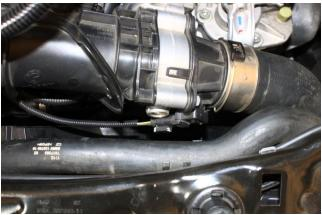
Locate the T-MAP sensor electrical connection at throttle body.
