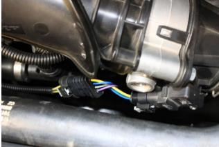
Route NM Power Module harness along the engine harness then underneath the throttle body up to the factory connector. Mate factory connector to Module connector and then Module connector to throttle body.
