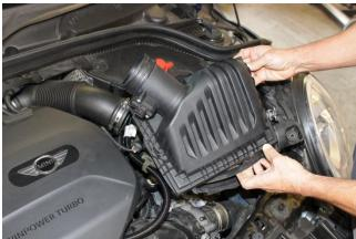
Lift out air filter box. NOTE: There are [2] pin mounts that sit
