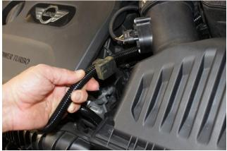
Disconnect rubber support for battery cable from air filter box.
