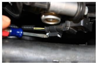
Using small screwdriver, back out grey locking clip.
