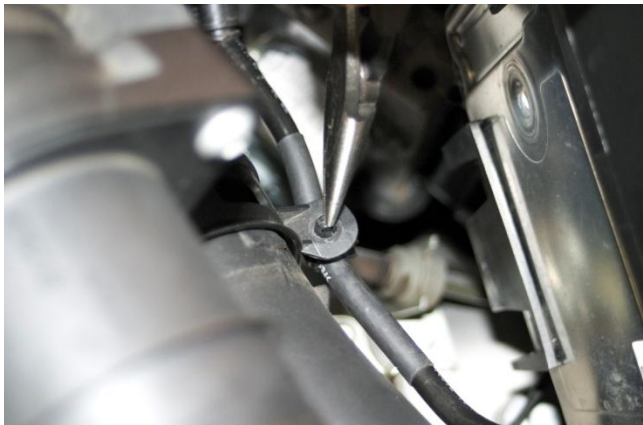
3. Separate brake booster line holder from fresh air intake hose. Use needle nose pliers to squeeze tabs and then push out holder.
