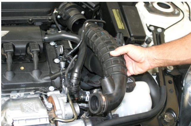
2. Remove OE turbo inlet hose: Use screwdriver to loosen clamp at turbo inlet and at air filter box.
