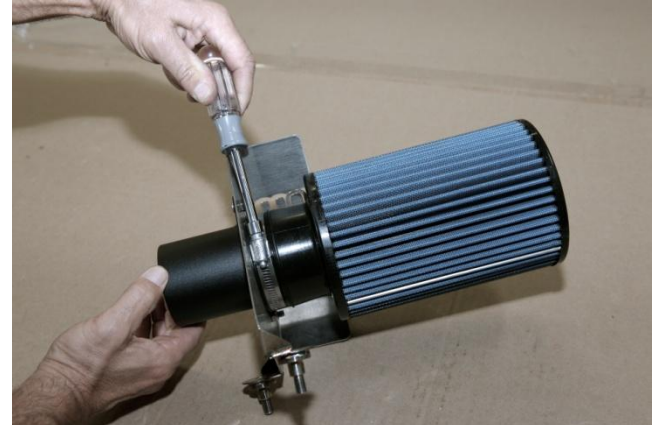
7. Using degreaser or contact cleaner and shop rag, clean inner mounting flange of NM filter. Install and tighten filter onto adapter pipe. Position NM logo on end of filter for proper reading orientation.
