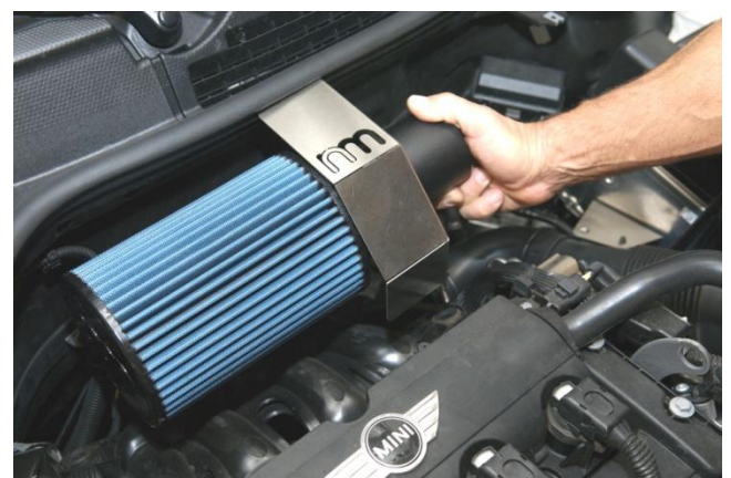
7. Using degreaser or contact cleaner and shop rag, clean inner mounting flange of NM filter. Install and tighten filter onto adapter pipe. Position NM logo on end of filter for proper reading orientation.
