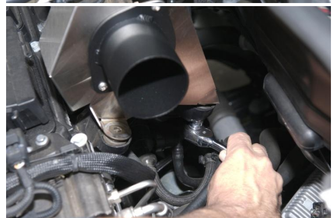
8. Install NM filter assembly unit onto factory air filter box mounts. NOTE: Make sure rubber grommets are still in place and not attached to bottom of the OE air filter box. From bottom side of mounts, install and tighten using supplied M8 washers and M8 lock nuts. [13mm socket or wrench]
