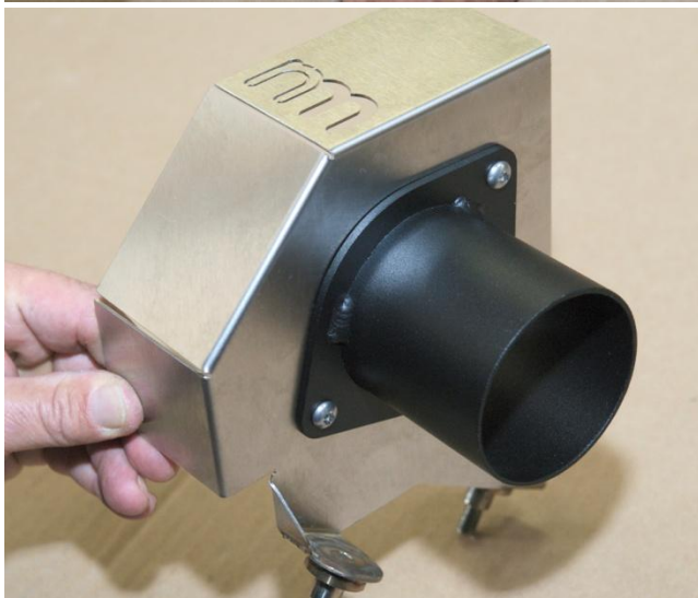
6. Install adapter pipe to NM stainless steel intake pipe bracket using supplied M6 x 16mm button head bolts and M6 nuts. [4mm hex key wrench / 10mm socket or wrench]
