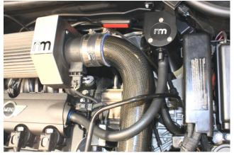
Using about 15" of supplied hose install from valve cover to bottom fitting on Catch Tank. Spray WD-40 or equivalent to ease installing hose onto fittings.
