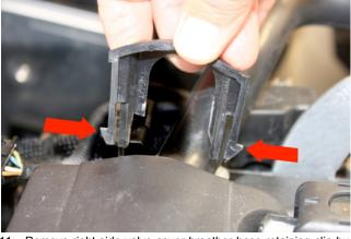
Remove right side valve cover breather hose retaining clip by squeezing lock tabs at the bottom, then pull up. 11.
