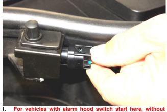
For vehicles with alarm hood switch start here, without switch proceed to step #8. Remove air intake tube or factory air box for easier access. Disconnect electrical connection by squeezing locking tab and then pull out.
