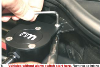
Vehicles without alarm switch start here. Remove air intake pipe or factory air box for easier access. Using M6x 16mm Button Head screw, washer and lock nut mount Catch Tank to top side of tab on plastic firewall
