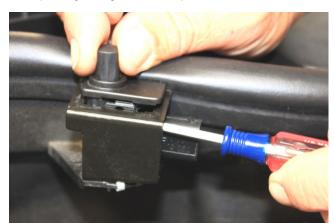
Between switch and mounting bracket there is locking tabs on each side, using a small screw driver push in to release.
