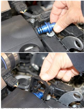
Lightly oil "O" rings on supplied billet fitting an install into breather port then reinstall factory retaining clip.
