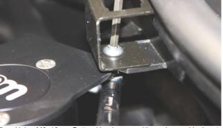
Using M6x16mm Button Head screw with washer and lock nut, 7. install in order; switch bracket, plastic mounting tab then Catch Tank bracket on bottom then washer and lock nut. Proceed to step #9.
