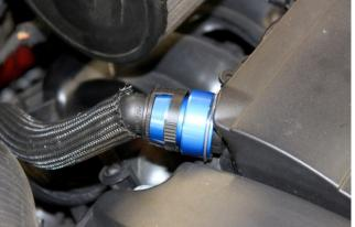
Disconnect breather hose at back left side of valve cover by squeezing locking collar. Lightly oil "O" ring on billet plug and install into valve cover port with locking spring clip facing outwards as pictured. Now re-install factory hose onto billet fitting.
