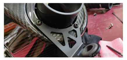
3. Pick up two more of the short bolts and add a washer to each. They can then be installed in the remaining two holes on the airbox.
