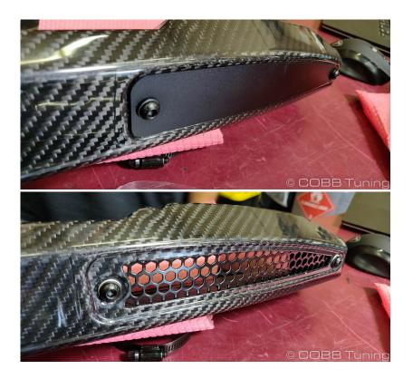
5. Use the provided foam tape to make a seal around the airbox lid. Make sure to stick to the provided flat area.
