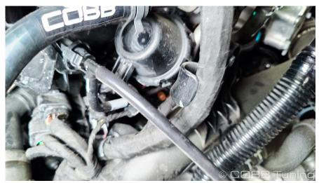
5. Slip the end of the silicon over the turbo intake.
