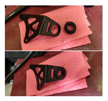
2. Next we're going to install the air filter adapter into the carbon airbox. To do so you'll slip it inside the airbox and poke it out the back. Using two of the supplied shorter allen bolts attach the bracket to the bottom and left side holes when facing it from the back.
