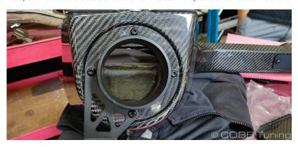
4. Looking at the back side of the airbox there is a removable panel. The factory panel allowed some air through this area to circulate in the engine bay so remove the two allen bolts if you'd like to keep this. If you're less worried about cooling the drivetrain you can close off this panel.
