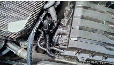
6. Now you should be able to pull the stock airbox and intake tube out of the car by popping the box off of the grommets that hold it in place. Lifting up in the back where the hose attaches the airbox and then rolling it towards you and out helps it drop out of the inlet box.
