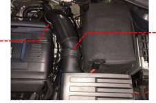
2 Disconnect the breather pipe from the turbo inlet pipe.
