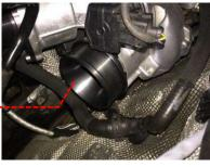
Pull the small vacuum pipe off the side of the airbox lid then remove the OE airbox lid by removing the 8 x T25 self-tapping screws. You will need to reuse these for the installation so keep them safe. Note: if you have a secondary air breather pipe on your airbox you will need to remove this also.
