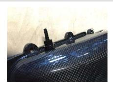
7 Install the new Revo carbon airbox lid using the 8 x T25 screws, removed earlier, and the rubber washers provided. Tighten to 3Nm. When tightening the lid ensure you do not apply excessive pressure. As you tighten each screw down you will feel them bite, once you feel it compress on the filter, stop. Note: over tightening of the lid will result in unnecessary damage and void your warranty.
