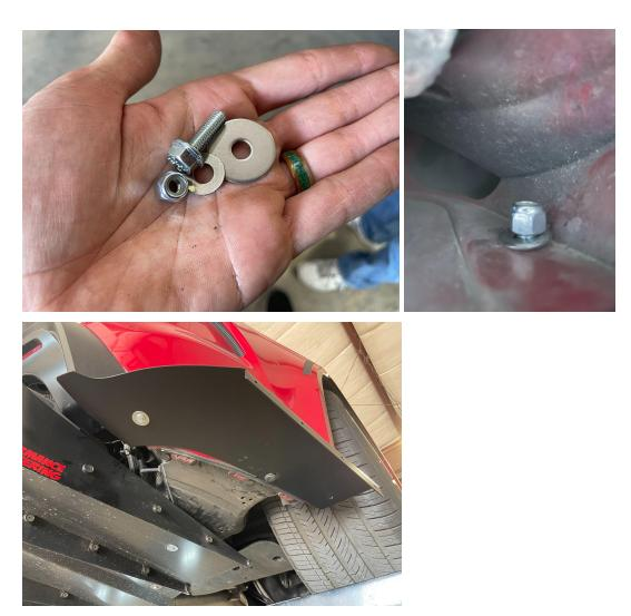
4.) Use your 1/4" drill bit to drill the remaining hole in the spat. Then install a M6 bolt at that location.
