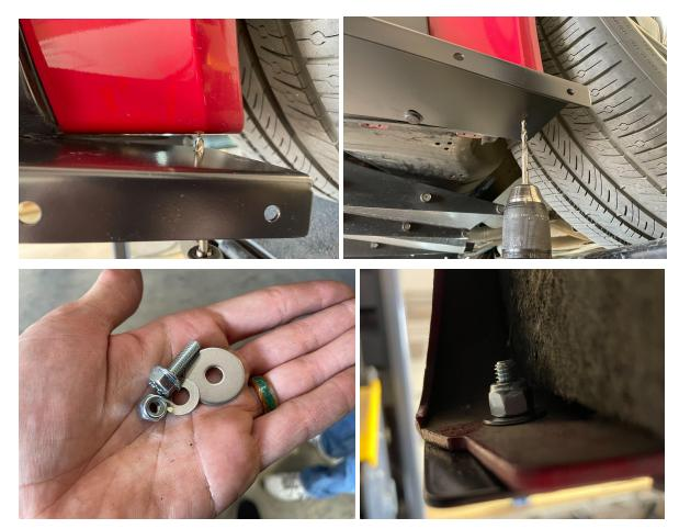
5.) Install your fin onto the spat with your ¼" hardware. Point the bolts inward with the countersunk washers underneath the heads and nuts on the inside. THIS IS VERY IMPORTANT: USE OIL ON THE THREADS OF THESE BOLTS WHEN TIGHTENING / LOOSING - IT IS REQUIRED ON STAINLESS STEEL BOLTS / NUTS!!!
