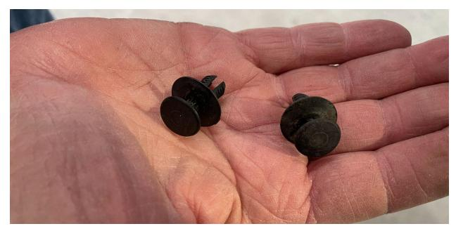
3.) Hold your spat up against the car. The fold for the bolt-on fin must be downward. "Pop" it onto the car with a pop clip at the center hole. Then install your M6 hardware into the OEM rearward hole with a large washer on bottom and small washer on top.
