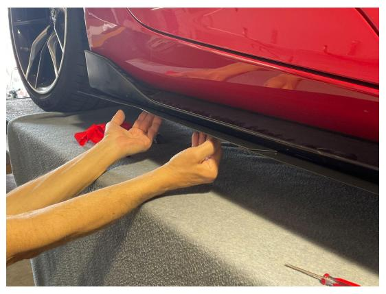
7.) Identify the 2 holes at the front of the side skirt. Drill through them into the car with a 7/64" drill bit - above them there are dimples in the car's body. Install the #8 screws with your phillip's head screwdriver.
