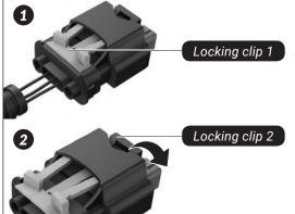
In the first step, the orange *locking clip* 1 is pulled out. Press the black *locking clip* 2, which functions as a lever for loosening the plug and pulling it out
