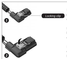
In the first step, the orange *locking clip* is pulled out. Press the orange *locking clip*, which functions as a lever for loosening the plug and pulling it out.
