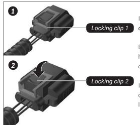
In the first step, the red *locking clip* 1 is pulled out. Press the black *locking clip* 2, which functions as a lever for loosening the plug and pulling it out.
