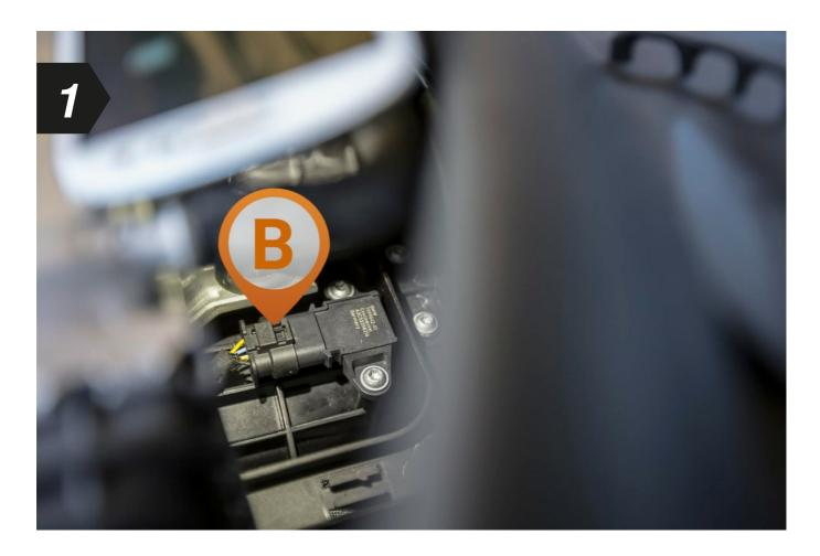
• To begin, locate the connection to the manifold absolute pressure sensor in your engine bay.
