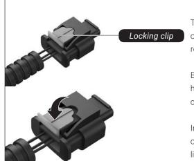
The first step involves pulling out the bright grey *locking clip*. Press down on the bright grey *locking clip*, which serves as a switch for releasing and removing the plug.
