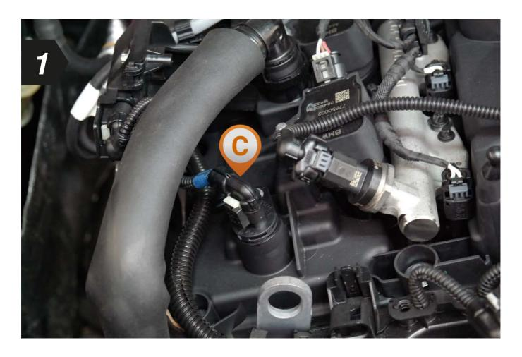
• To begin, locate the connection to the camshaft sensor in your engine bay.
