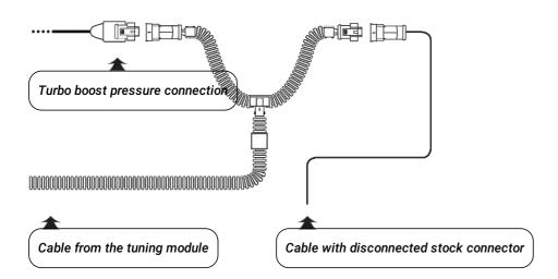
• Disconnect the plug from turbo boost pressure sensor.
