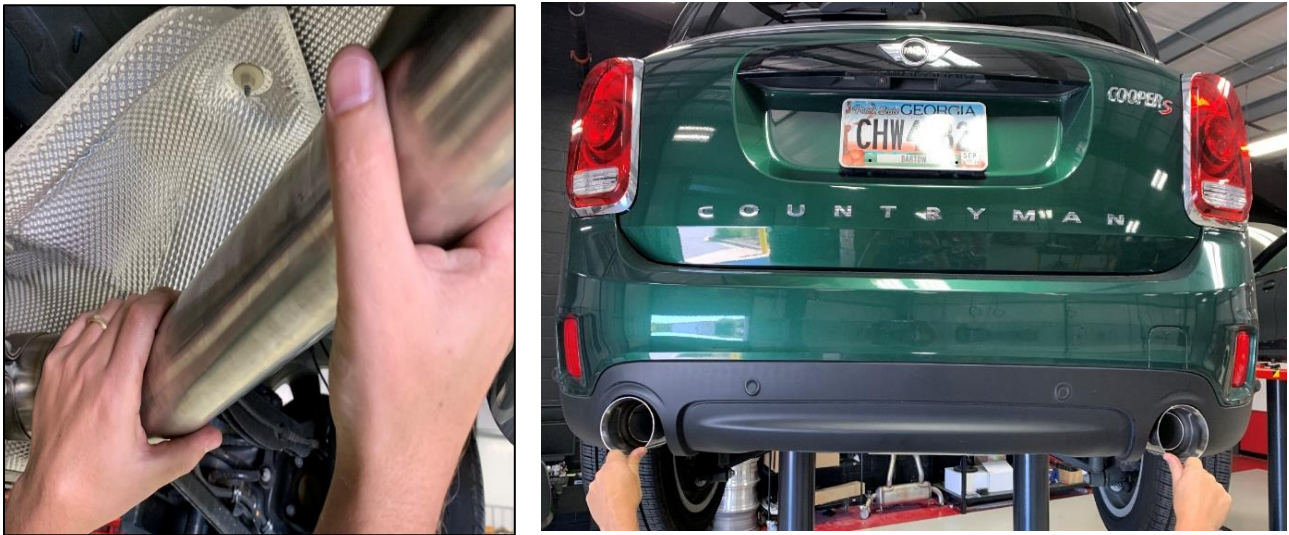
Figure 11: Aligning the Exhaust System
