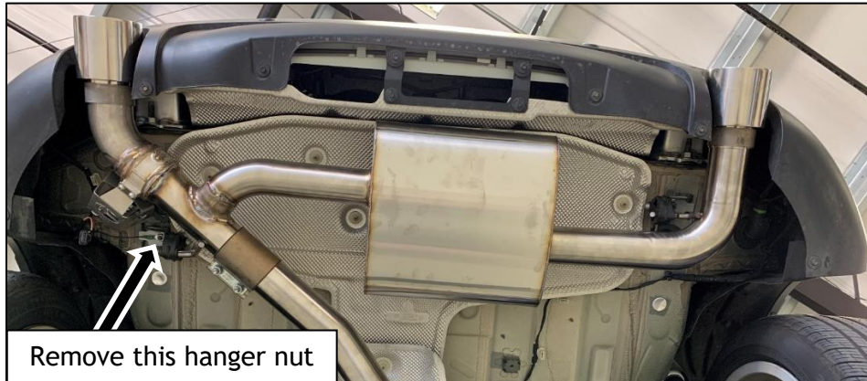
Figure 30: Hanger Ground Location
