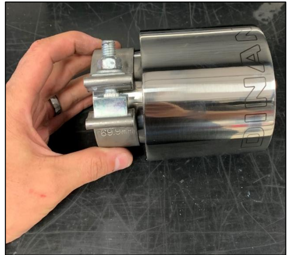
Figure 9: Tip Clamp Location
