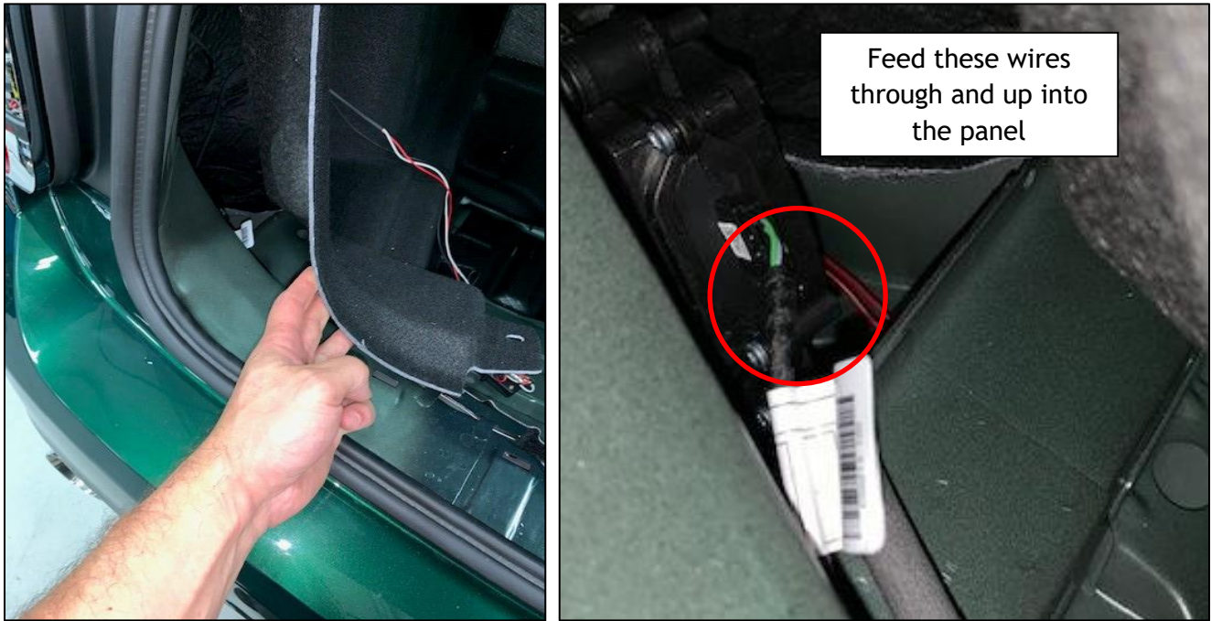
Figure 17: Connector Plug Routing
